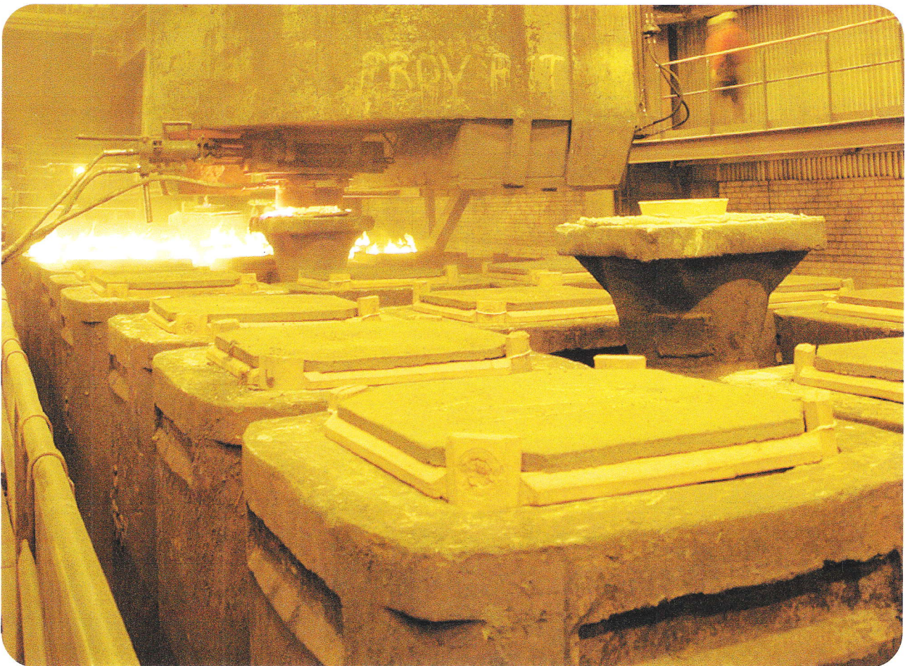
Vallak® Hot-Top with FERROX Anti-Piping Board
